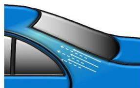
Mix Standocryl VOC Performance Pro Clear K9590, Standocryl VOC Xtreme Plus Clear K9600 or Standocryl 2K Classic Pro Clear K9070 according to the TDS. Overcoat the appropriated Standox basecoat quality with ready-to-spray Standocryl VOC Performance Pro Clear K9590, Standocryl VOC Xtreme Plus Clear K9600 or Standocryl 2K Classic Pro Clear K9070. Fade out the clear in staggered coats with reduced pressure onto the sanded area and till the edge of the polished area.
